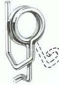
Figure 1. Hook for engagement over the archwire is replaced by two 90-degree bends. Spring formed of .014" wire.
