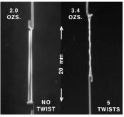
**Figure 2.** Untwisted <sup>5</sup>/<sub>16</sub>" light elastic (left) pulls 2.0 ozs. when extended 20 mm. When twisted 5 times, pull increases to 3.4 ozs. (right).
